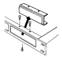
3. Mounting the Tuner Unit into the Diversity Receiver and tighten 2 screws (provided).
