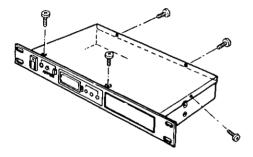
2. Remove 3 screws and remove the blank panel (TUNER 2 side).
